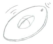
Table top anti-wave device that picks up unwanted sound in its microphone and sends the opposite frequency to counter it
