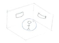
Speakers set up on each wall of a room using phasing to create a central bubble of sound in the room surrounding the user.
