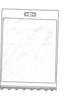
This concept uses room mapping and motion tracking sensors at the top of the product to sense where you are in the room and focus the music directing the sound at where you are.
