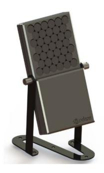
An on board signal processor conditions the audio from your iPhone, iPod, iPad, computer or any other source. The sound can only be heard by someone standing in the Soundlazer's path. Like a laser, the parametric array sends the audio signal over a ultrasonic beam which can also be bounced off of walls, statues or any other hard object to make the sound appear to be coming from another direction.
