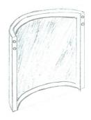
Curved shape to encapsulate the head with sound, as well as giving support for the tickness of the concept.
